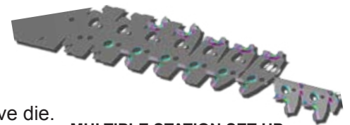
MULTIPLE STATION SET-UP
